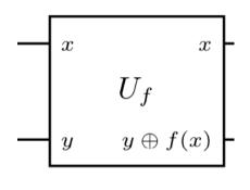
In the Deutsch-Jozsa case, our oracle takes an unknown function f(x) and wraps it in a unitary gate so that it is now "quantum compatible".
