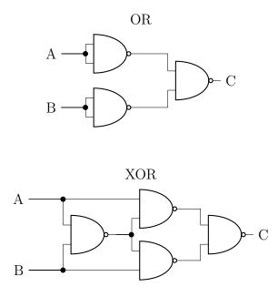
The idea of functional completeness is extremely important in computing. If we want to make a computer, we must make physical circuits that perform these logical operations. If we have a functionally complete set of operations, {NAND} for example, we only need to know how to make that specific circuit, and then can make any operation necessary by combining the gates in different ways.
